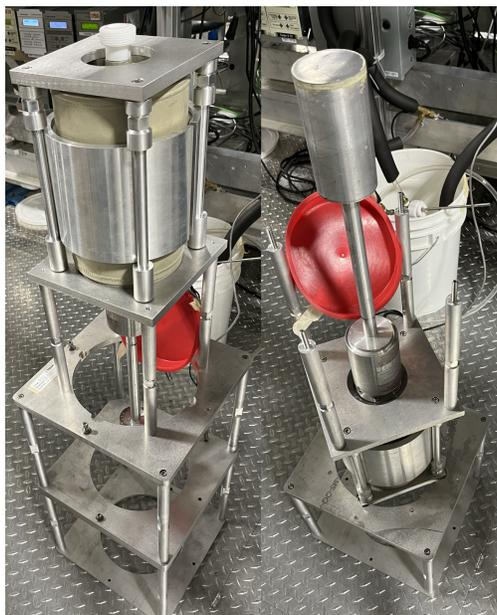
**Figure 6.13:** The  $\gamma$ -ray detector stands for detector maintenance and calibrations. (left) The detector is mounted in an upright orientation which allows for access to the LN2 dewar and enough space under the detector for a calibration source. (right) The detector is mounted in an inverted orientation which allows access to the detector window and the preamplifier electronics.
