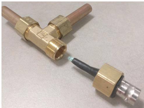
**Figure 6.16:** The temperature sensitive green LEDs (P/N HLMP1790, Digikey P/N 516-1310-ND) used as temperature sensors in the LN<sub>2</sub> system. After soldering the leads, they are coated in a black moldable glue (Sugru™).
